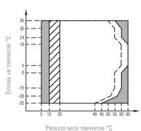
Operating range with heat pump with possible limitation and protection
